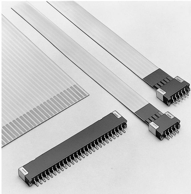
**The FFS series connectors are designed for surface mounting (SMT) and to meet the demand for high-density packaging. They are miniature connectors with a height of only 2.8mm. Their high contact pressure eliminates fretting corrosion and ensures secure connections. Low insertion force make connection easy.**
