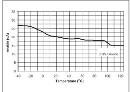
Figure 17. ENABLE Current vs Temperature at V<sub>EN</sub>=16V
