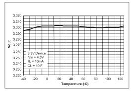
Figure 10. Output Voltage vs Temperature at  $I_{LOAD}$ =10mA
