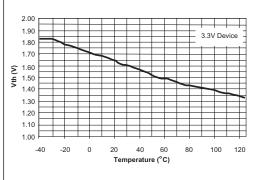
Figure 18. ENABLE Threshold vs Temperature
