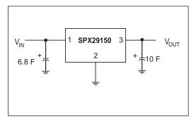
Figure 19. Fixed Output Linear Regulator
