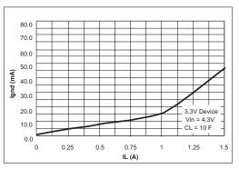
Figure 5. Ground Current vs Load Current
