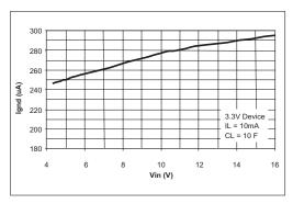
Figure 6. Ground Current vs Input Voltage
