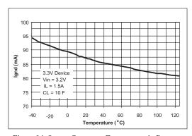
Figure 14. Output Current vs Temperature in Dropout at  $I_{\rm LOAD}$ =1.5A
