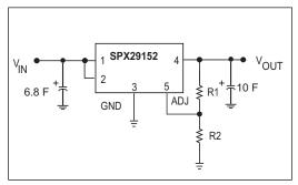
Figure 20. Adjustable Output Linear Regulator
