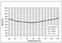
Figure 9. Ground Current vs Temperature at  $I_{LOAD}$ =10mA
