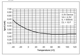
Figure 11. Ground Current vs Temperature at  $I_{LOAD}$ =500
