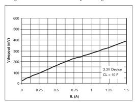
Figure 8. Dropout Voltage vs Load Current
