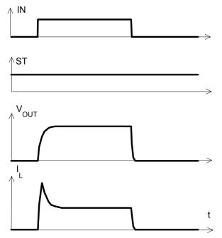
The initial peak current should be limited by the lamp and not by the initial short circuit current  $I_{L(SCp)}=14$  A typ. of the device.
