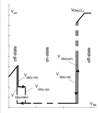
IN = high, normal load conditions. Charge pump starts at  $V_{bb(ucp)} = 5.6 \text{ V}$  typ.
