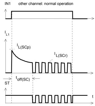
Heating up of the chip may require several milliseconds, depending on external conditions ( $t_{off(SC)}$  vs.  $T_{i,start}$  see page 12)
