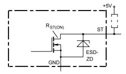
ESD-Zener diode: 6.1 V typ., max 5.0 mA;  $R_{ST(ON)}$  < 380  $\Omega$  at 1.6 mA, ESD zener diodes are not to be used as voltage clamp at DC conditions. Operation in this mode may result in a drift of the zener voltage (increase of up to 1 V).
