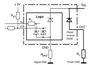
$R_{GND} = 150 \Omega$ ,  $R_{I} = 3.5 k\Omega$  typ,
