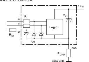
$V_{Z1} = 6.1 \text{ V typ., } V_{Z2} = 47 \text{ V typ., } R_{I} = 3.5 \text{ k}\Omega \text{ typ.,} \\ R_{GND} = 150 \ \Omega$
