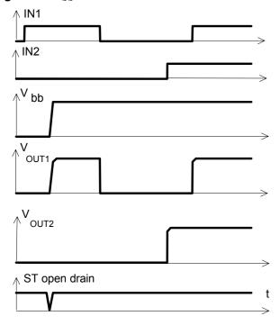
Figure 2a: Switching a lamp:
