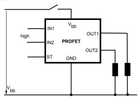
For an inductive load current up to the limit defined by  $\mathsf{E}_{AS}$  (max. ratings see page 3 and diagram on page 10) each switch is protected against loss of  $\mathsf{V}_{hb}$ .
