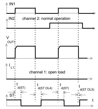
The status delay time td(STOL4) allows to distinguish between the failure modes "open load in ON-state" and "overtemperature".
