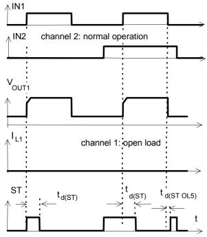
$t_{\text{d(ST\ OL5)}}$  depends on external circuitry because of high impedance
