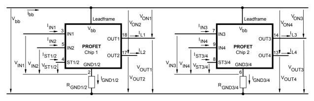
Leadframe (V<sub>bb</sub>) is connected to pin 1,10,11,12,15,16,19,20
