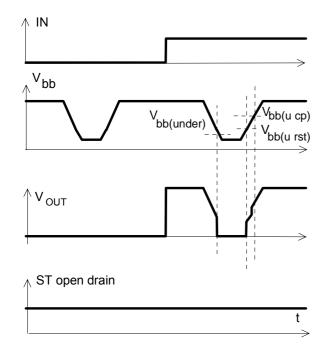
Figure 6b: Undervoltage restart of charge pump
