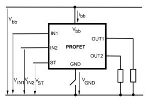
Any kind of load. In case of IN = high is  $V_{OUT} \approx V_{IN} - V_{IN}(T+)$ . Due to  $V_{GND} > 0$ , no  $V_{ST} =$  low signal available.
