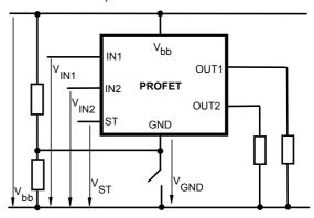
Any kind of load. If  $V_{GND} > V_{IN} - V_{IN(T+)}$  device stays off Due to  $V_{GND} > 0$ , no  $V_{ST} = low$  signal available.
