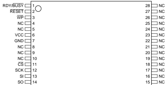
TSOP Top View Type 1
