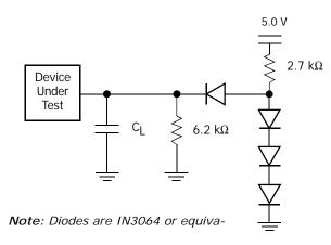
Figure 7. Test Setup
