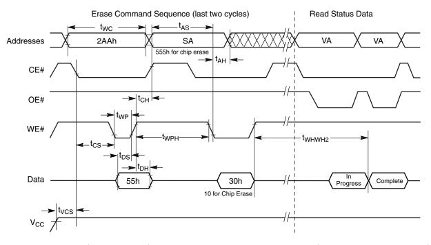
Note: SA = sector address (for Sector Erase), VA = Valid Address for reading status data (see "Write Operation Status").
