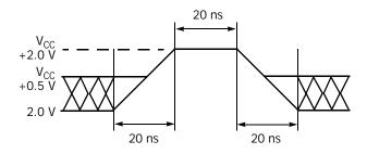
Figure 6. Maximum Positive Overshoot Waveform
