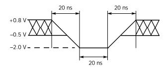
Figure 5. Maximum Negative Overshoot Waveform
