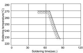
In case of repeated soldering, the accumulated soldering time must be within the range shown above.
